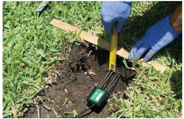
Soil moisture sensor. Photo courtesy of Bernardo Cardenas
