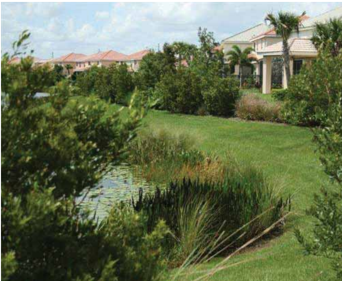
A 10-foot-wide maintenance-free zone protects a water body from fertilizer and pesticide runoff.
